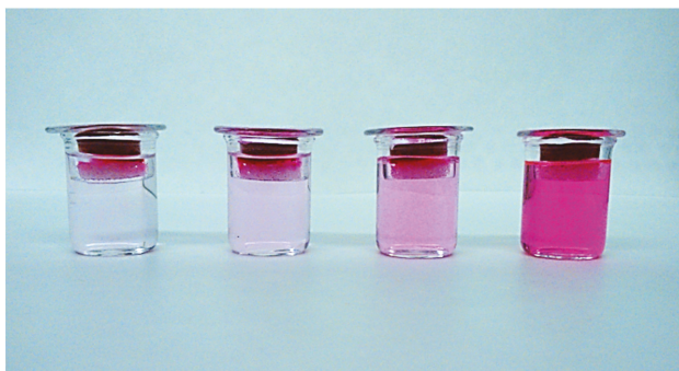
Figure 6. Equipment employed to study the release of rhodamine B in physiological conditions. The photo refers to different release times.
