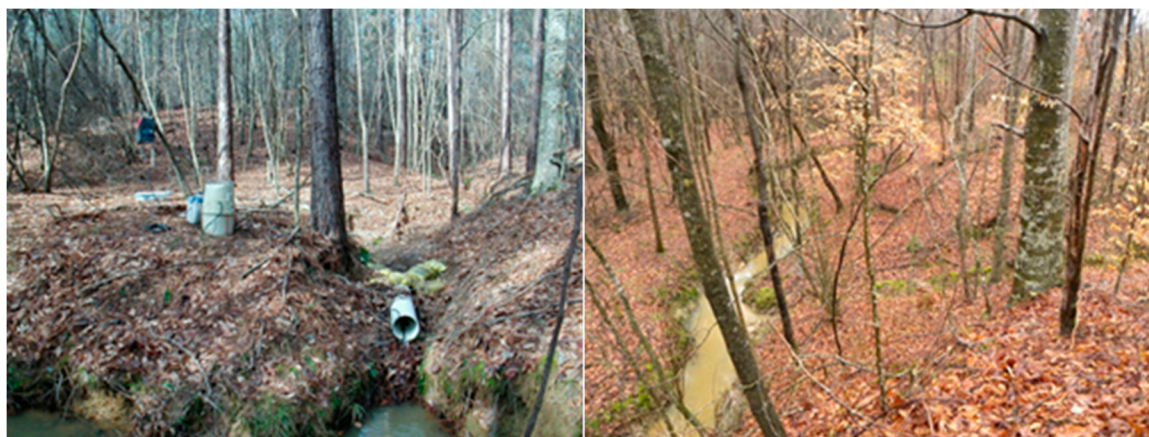
Figure 2. Left: Gauged reference stream with a 254 mm diameter pipe, ISCO sampler, and flowmeter. Right: Ephemeral stream flowing during storm event.
