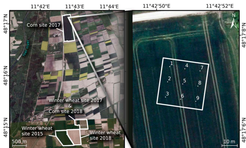
Figure 1. Munich-North-Isar test sites overview (left) and exemplary 2017 simulated 30 × 30 m corn EnMap-pixel with 9 ESUs (right).
