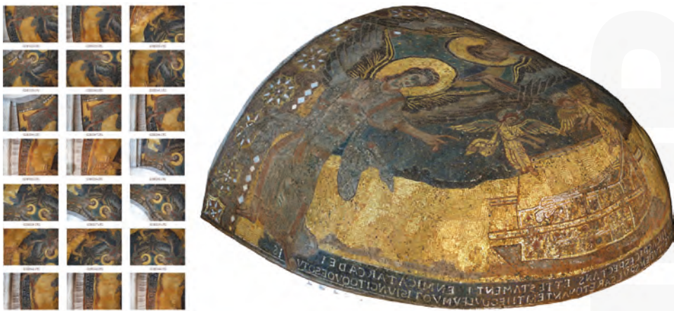
Figure 4. Point cloud from a set of 2D poses reconstructed via dense-image matching using the software ContextCapture v 4.4.6, Bentley Systems, Exton, United States [37].
