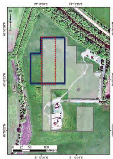
Figure 3. Area covered from the different techniques: Grey and blue polygons indicate the areas covered from the geophysical surveys (magnetic and GPR survey, respectively), the red polygon indicates the area covered from the ground spectroradiometric measurements while the whole area is covered by the GeoEye image (no polygon used) (Latitude: 46^{\circ}56'24.36'' ; Longitude: 21^{\circ}12'32.67'' , WGS84).
