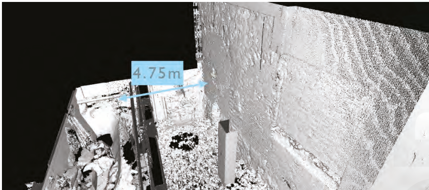
Figure 5. Documentation of the main portion of the circus outer wall still standing; laser scan including a small remnant of the inner wall found in a private basement, providing the height of the wall in this point of the structure, and its distance from the inner one.
