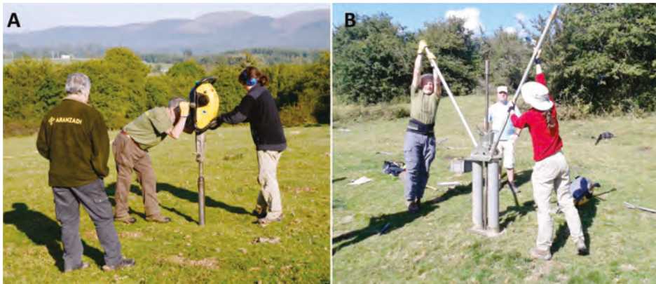
Figure 2. (A) Photograph of the power auger (Cobra TT engine) used for drilling; (B) Photograph of ARANZADI and MOLA team removing the gouge manually.
