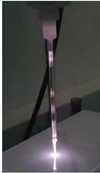
Figure 1. A photo of the atmospheric-pressure plasma jet. The substrate is a wooden plate at a floating potential.
