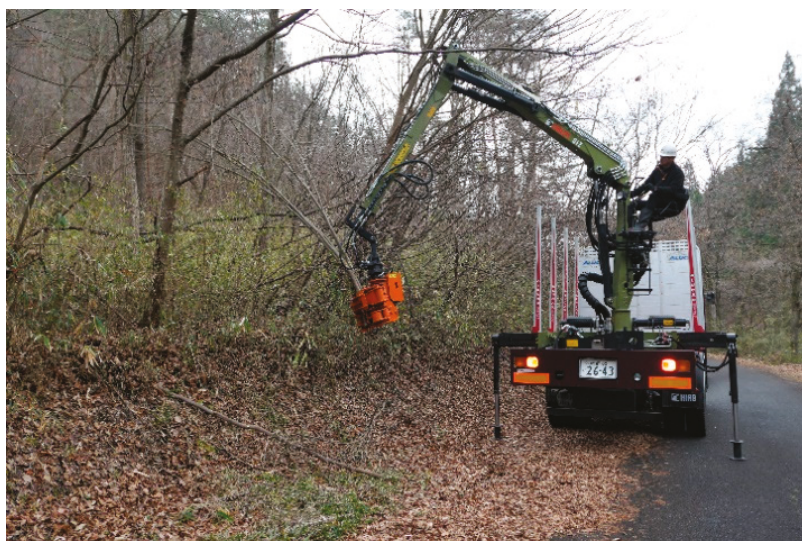
Figure 4. Harvesting experiment with a truck-mounted multi-tree felling head.
