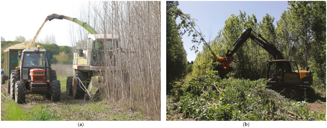
Figure 1. Mechanized harvesting systems on poplar rotation coppice plantations: (a) Forage-Based Harvesting System (FBHS); (b) Shear head-Based Harvesting System (SBHS).
