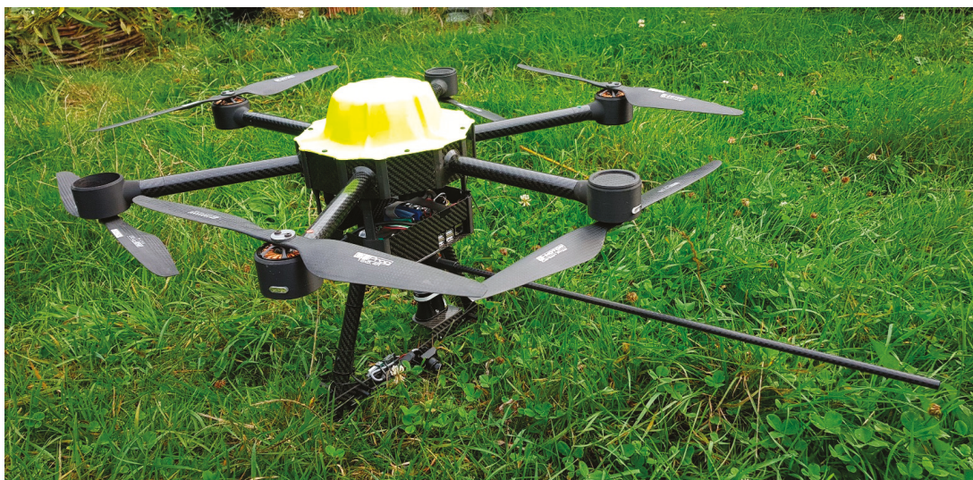
Figure 2. Picture of the PROTECT FOREST drone with the sensor system and capillary.
