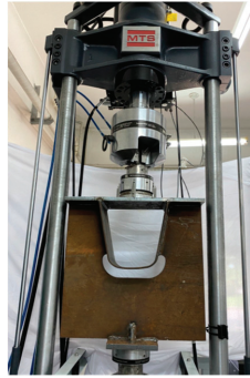
Figure 9. Fatigue loading of specimens.
