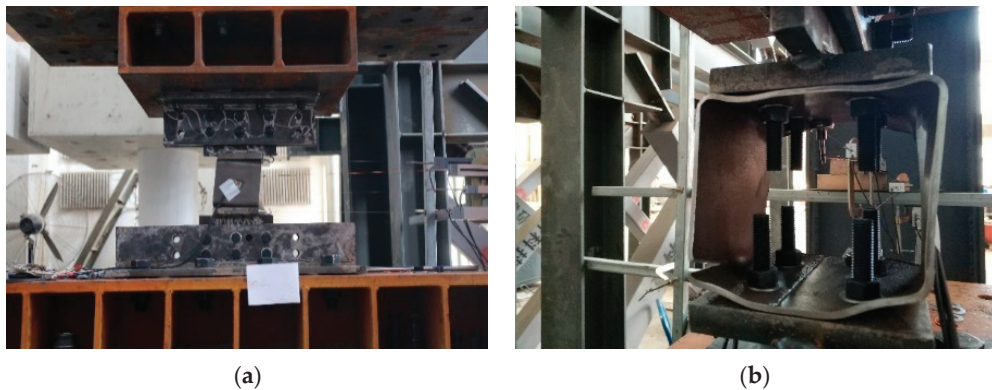
Figure 8. Failure modes of the bolted steel tube dampers: (a) corner of 150-D1 warping; (b) steel tube end of 150-D1 tearing.
