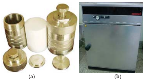
Figure 2. Images of the Teflon-lined stainless steel autoclaves (a) and an oven with temperature control (b) typically applied for the hydrothermal generation of CPs.
