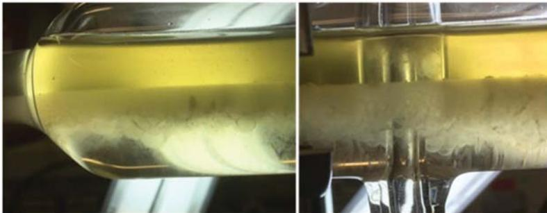
**Figure 14.** Side view of the laboratory settler (DN35, 175 mL hold-up. DN: diameter nominal) during continuous settling operation (300 s residence time). The image shows the inlet area (**left**) and the heavy phase outlet (**right**).
