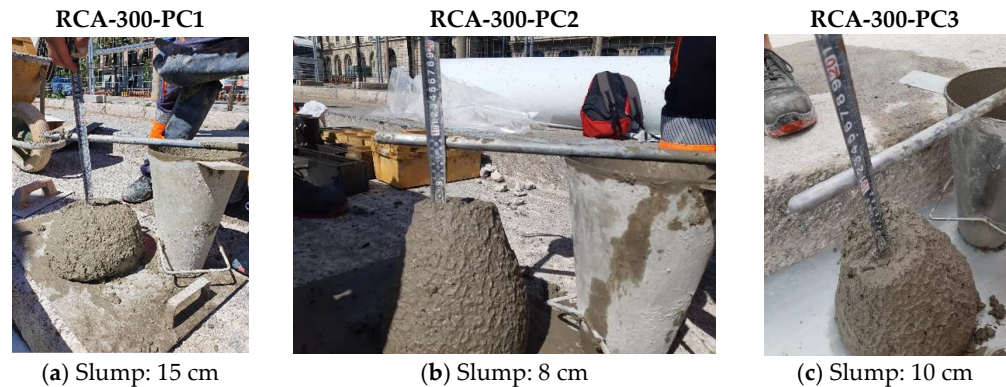
Figure 5. On-site slump test determination.
