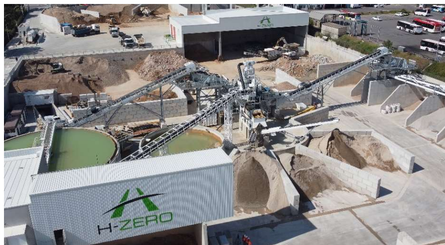
Figure 1. CDW recovery plant to water-washed recycled aggregate [35].
