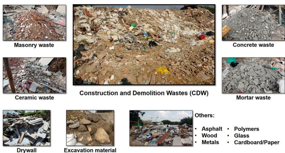
Figure 1. Actual composition of the sample of CDW utilized in this research. Site for final disposal of waste located in the city of Cali, Colombia.
