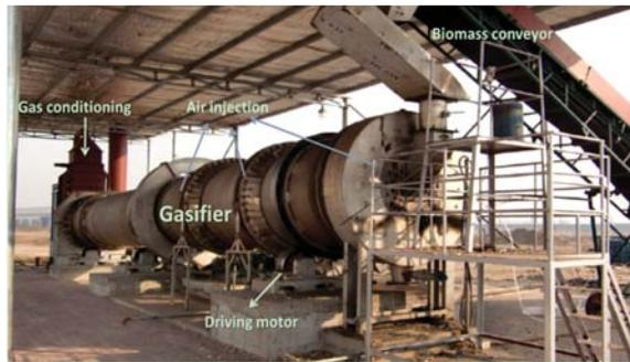
Figure 3. A view of the 1.5 MW<sub>th</sub> biomass gasification system.
