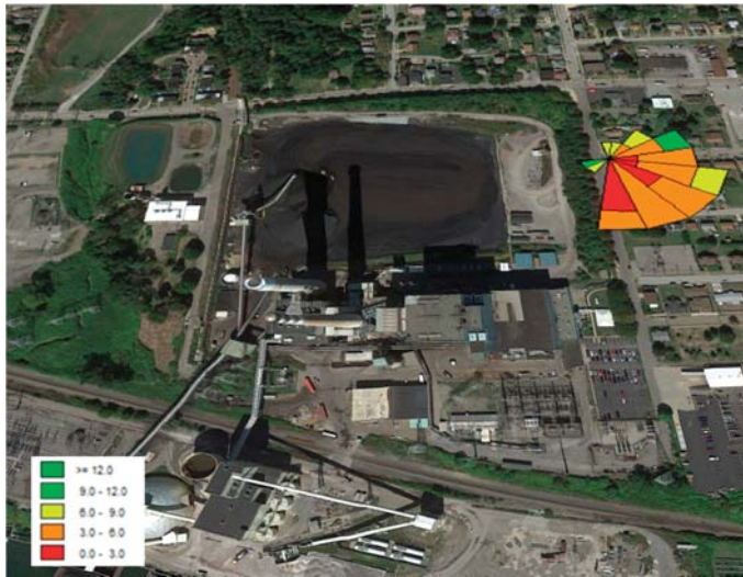
Figure 6. Wind rose created for PM_{2.5} concentrations measured at Station 1. Green colors represent the highest concentrations of particulate matter while the orange and red colors represent lower concentrations of particulate matter, as shown in the legend. Units of particulate matter concentration are \mu\text{g m}^{-3} . The upper side of the wind rose represents North. The length of the wind rose vectors represents average wind speed, where the longer vectors represent a higher average wind speed.
