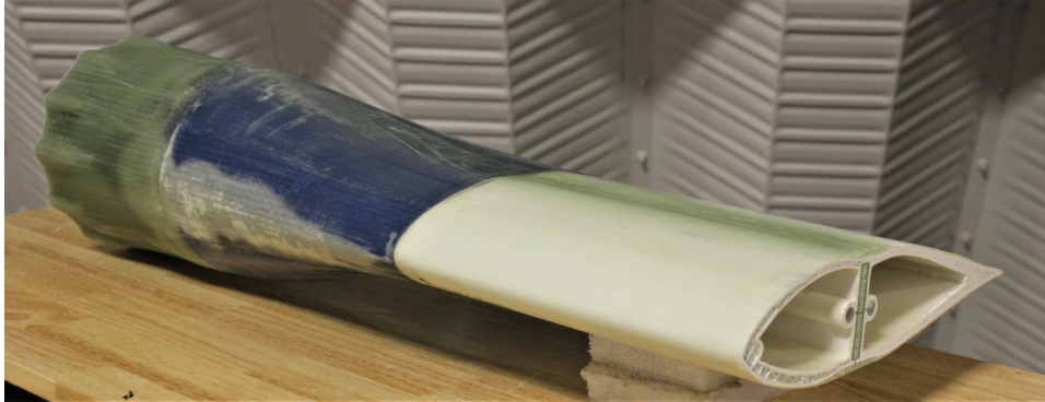
Figure 10. The final finished blade section with visible out-of-plane waves stemming from the root inserts and the delamination along the leading edge of the transition region.
