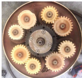
Figure 24. Spur gear failure in a ball-milling machine.
