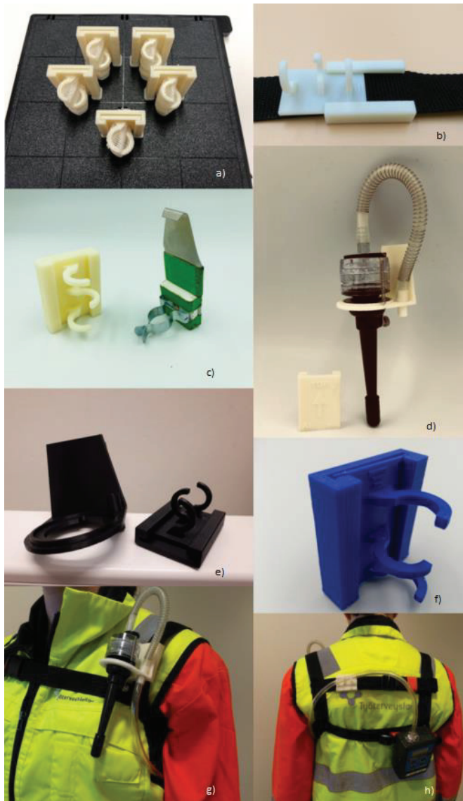
Figure 3. (a) Five hose holders with support structures in the printing bed; (b) sliding the slider into the sheath; (c) new (white) and old hose holder (green and metal original cyclone sampler assembly); (d) cyclone sampler assembly with the redesigned holder; (e) black hose holder clip and cyclone sampler clip printed as part of supply chain testing; (f) blue hose holder clip printed with Lulzbot Mini; (g) sampler system with cyclone sampler clip from the front; (h) harness with sampler system from the back.
