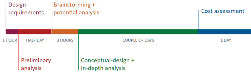
Figure 2. Example of timeline for a common design process involving additive technologies in the field of machined parts.
