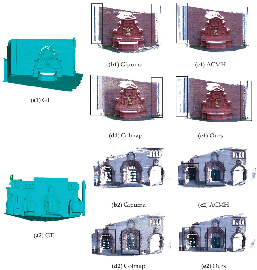
Figure 11. The comparison of reconstructed point clouds with the Strecha dataset. (a1,a2) are the ground truth meshes of the Fountain and Herzjesu datasets, respectively. (b1–e1) and (b2–e2) are generated by Gipuma, ACMH, Colmap, and the proposed method with the Fountain and Herzjesu datasets, respectively.
