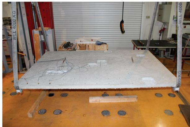
Figure 2. Suspended plate with discrete damages.
