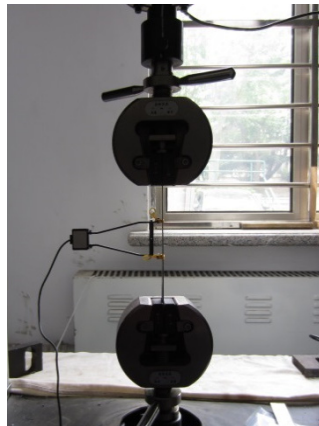
Figure 2. Tensile test of BFRP laminates.
