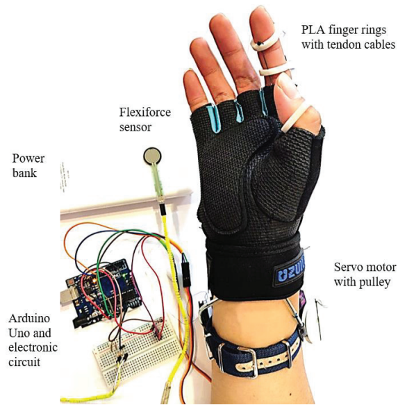
Figure 17. Pinch assistant prototype.
