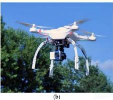
**Figure 1.** A Xiaomi Yi action camera; **(a)** in improving phase; **(b)** on a 3-axes gimbal on an Unmanned Aerial Vehicle (UAV).
