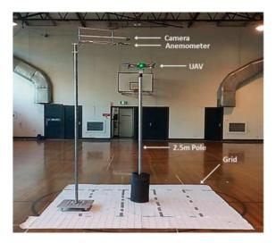
Figure 3. Set up of the multi-rotor UAV and airspeed measuring pole for aerodynamics test.
