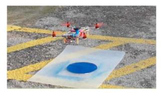
Figure 9. Smart-drone prototype and corresponding landing pad.
