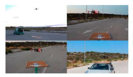
Figure 8. UAV landing on a moving platform.
