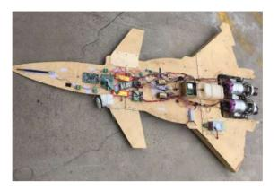
Figure 1. The thrust-vectored tail-sitter unmanned aerial vehicle (UAV).
