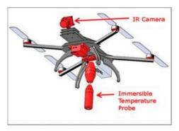
**Figure 1.** Overall design concept. The UAS flies over the thermal water plume using its navigational (auto-pilot) capabilities. Key components carried by the UAS include an IR camera for thermal imaging of the water surface, an immersible probe that can be lowered and raised to measure the vertical temperature profiles below the water surface, and a controller that stores the data.
