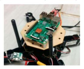
Figure 8. Onboard computer module.
