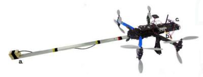
**Figure 13.** Close up of chosen Unmanned Aerial Vehicle (UAV): X8+ from 3DR. Important components are highlighted on the picture. (a) Sensor head with an 1.1 m aluminium boom; (b) compainion computer: Raspberry Pi 2; (c) sensor body.
