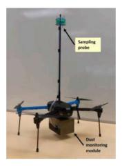
**Figure 2.** Physical configuration of the multi-rotor UAV with the sampling probe and dust monitoring module attached.
