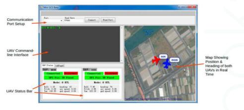
Figure 13. Graphic user interface (GUI) of Mini GCS.
