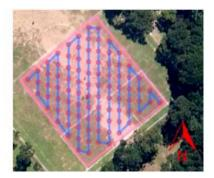
**Figure 7.** Example of generated path following magnetic north, with 5 m spacing between samples. The pink area is the region of interest, the blue lines are the expected path to be followed and the red circles are the discrete waypoints to visit.
