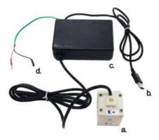
**Figure 1.** The developed sensor exposing the connectors. (a) The sensor core; (b) serial connector to acquire the data; (c) the Printed Circuit Board (PCB) protected by a small plastic case; and (d) power connectors.
