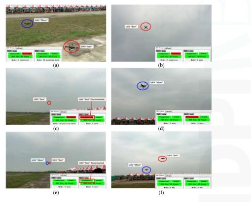
**Figure 22.** A rundown of flight test (a) Pre-takeoff setup of flight test; (b) UAV "Son" starts the mission; (c) "Son" is out of radio range and communication with it is lost; (d) UAV "Mom" is deployed to the relay position; (e) Communication with "Son" is re-established after being relayed through "Mom"; (f) "Mom" and "Son" return to launch position; the mission is completed.
