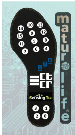
Figure 3. Location of the piezoelectric sensors on the insole.
