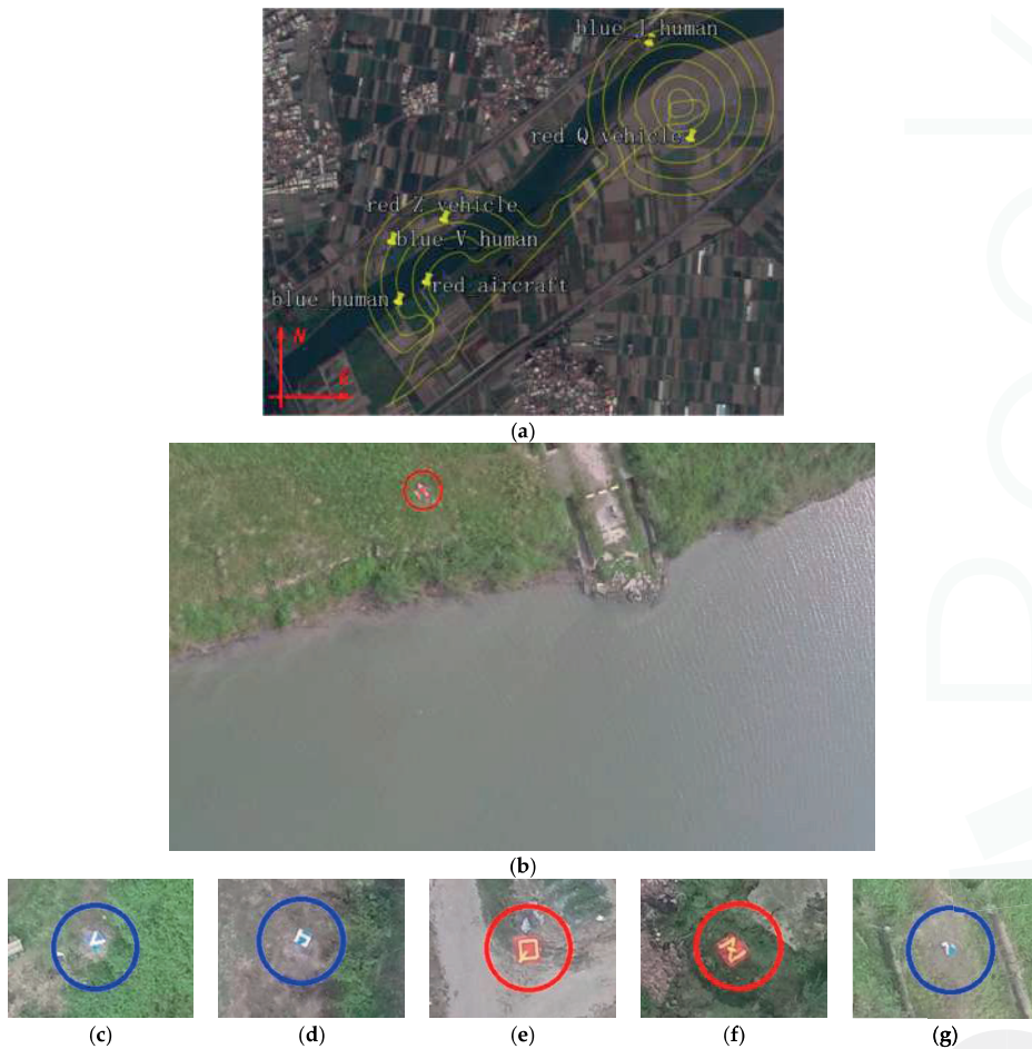
Figure 21. (a) The locations of six simulated targets; (b) the original image saved by the identification program with target drone; (c) designed target (blue board with letter V) represents an injured person; (d) designed target (blue board with letter J) represents an injured person; (e) designed target (red board with letter Q) represents a crashed car; (f) designed target (red board with letter Z) represents a crashed car and (g) designed target (small blue board) represents an injured person. The board was blown over by the wind.
