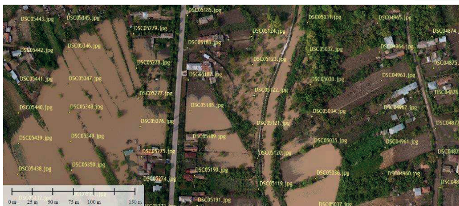
Figure 7. Image created from acquired images (with yellow ID) without overlapping or gaps. The image was generated with Agisoft Photoscan Professional Edition ( www.agisoft.com ).
