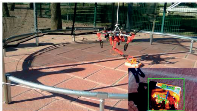
Figure 8. Robot grasping an object. The camera's view is given in the inset. The green rectangle is the tracked moved window.
