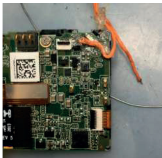
Figure 12. Modification of the GoPro buttons to PWM-controlled relay switch.
