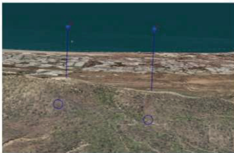
(b) augmented video (AR tool) from position A. Occluded targets are easy to locate using the virtual beacons.
