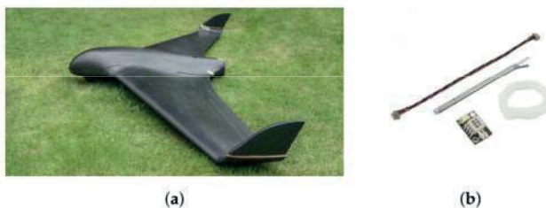
Figure 13. Sensor and UAS platform utilized in experiments. (a) UAS SkyWalker X8, (SkyWalker Technology Co., Ltd, Wuhan, China) with carbon fiber frame equipped with a 12 \times 6 prop with 2 \times 20 g servomotor; (b) Digital airspeed sensor utilized in experiments which contains a 4525DO sensor (TE Connectivity Ltd., Schaffhausen, Switzerland) which enables a resolution of 0.84 Pa [33].
