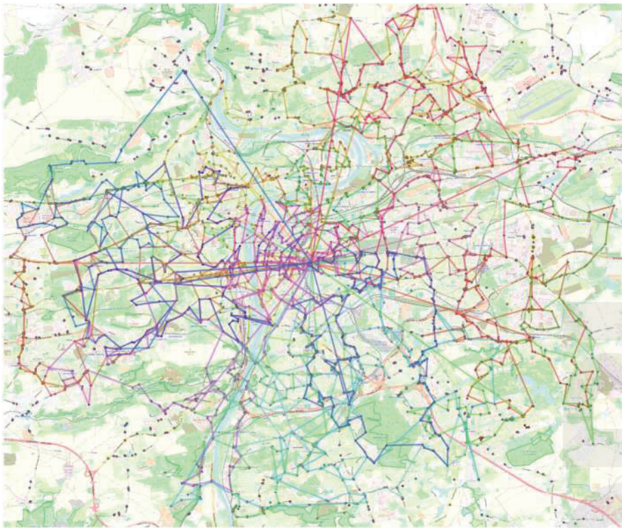
Figure 6. Planned trajectories for 20 UAVs tasked to monitor 3506 locations in Prague. Each location is required to be monitored by 3 different sensors giving 10,518 sensor tasks in total. DivPlan reached coverage of 64%.
