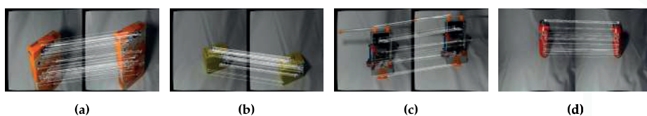
Figure 3. Sequential association of features to compute their inter-frame visibility. (a) Whooopies box 640 \times 480 ; (b) Gena box 640 \times 480 ; (c) Drilling tool 640 \times 480 ; (d) Coke 1280 \times 720 . Then, following Algorithm 1, the visibility between non-sequential frames is computed.
