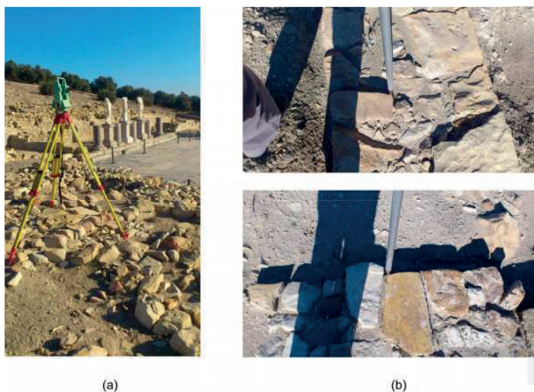
Figure 4. Assessing spatial resolution: (a) Measuring using the total station; and (b) Samples of spatial details of the ground measurements.
