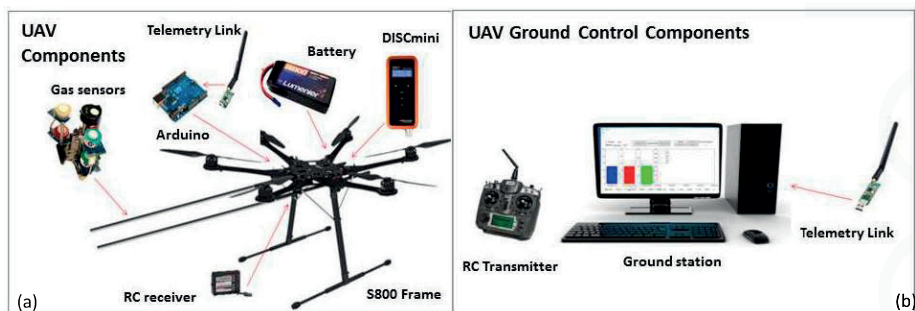
Figure 1. (a) Unmanned aerial vehicle (UAV) system components including gas sensors, DISCmini, Arduino MEGA 2560, battery and RC receiver; (b) UAV Ground Control Components for both manual (using RC transmitter) and autonomous (using PC) operations.
