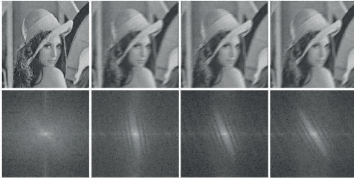
Figure 1. Figures from left to right are: original image with no motion, 20°, 40°, 60° movement in the horizontal direction. The figures blew are their corresponding spectrum.
