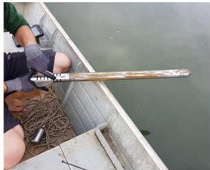
Figure 9. Picture of GraviProbe (GP) after deployment.
