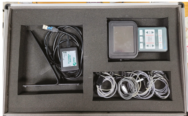
Figure 2. Surface EMG 4-channel wired instrument (MyoTrace 400).
