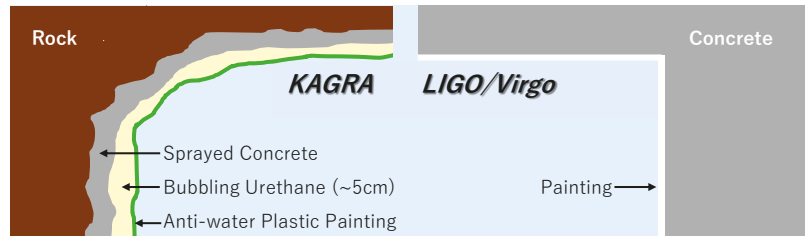
Figure 14. Schematic view of the walls in the experimental sites of KAGRA and LIGO/Virgo.
