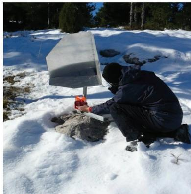
**Figure 19.** One of the small Corner Reflectors deployed over the landslide lower unit in order to fix up the vegetation and snow problems. The operator is holding a surveying circular prism, which is observed from a reference point with a Total Station, for validation purposes.
