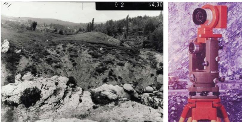
**Figure 4.** Left: example of a  $6 \times 8$  cm glass plate photograph of landslide toe taken from the Vallcebre Torrent. Right: Wild P32 camera for terrestrial photogrammetry over a theodolite, which was used for the landslide toe monitoring between 1987 and 1992.
