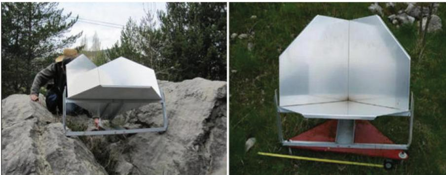
**Figure 15.** Corner Reflectors (CRs) used for DInSAR monitoring at the Vallcebre landslide [6]. Examples of installation on a big rock block (left) or directly over the terrain (right).
