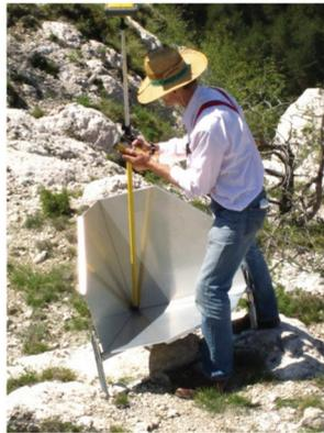
**Figure 23.** Cross-checking between techniques: every GPS campaign included the CRs (CR\_2 in the picture) and the top of the boreholes where the wire extensometers and/or the inclinometers were installed.
