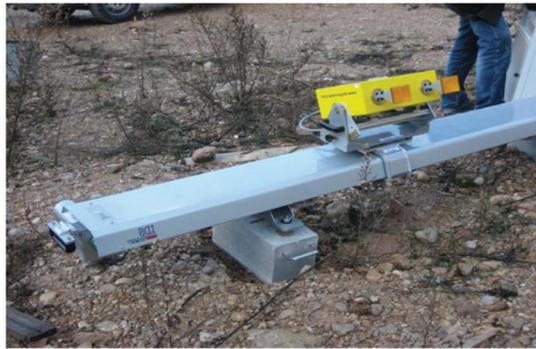
**Figure 18.** Picture of the IDS GBSAR system. The synthetic aperture is obtained through the movement of the radar sensor (yellow box) along the rail.
