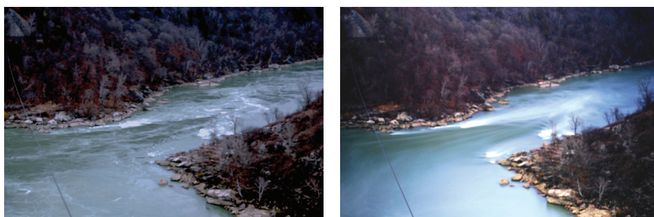
Figure 1. Two images of the same Niagara Falls downstream flow. The left image is an exposure of 1/2 sec, while the right hand image is exposed for 50 sec. Note the flow features visible in the right hand image (stream lines, bow waves, standing waves, vortices, etc.) that are not clearly visible or simply invisible in the left image due to the “noise” of local fluctuations.
