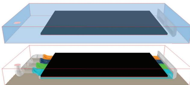
**Figure 3.** Outer faces of the calculation domain: top and sides faces are treated as pressure boundary and the bottom as adiabatic wall.
