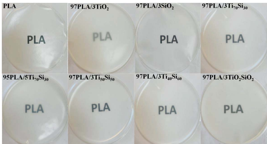
Figure 9. Photographs of films prepared from PLA, PLA/TiO 2 , PLA/SiO 2 , PLA/Ti x Si y , and PLA/TiO 2 SiO 2 composites (250 ± 4.68 μm thickness).
