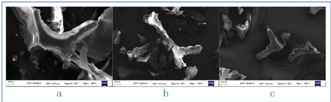
Figure 7. Microscopic morphology of PUF powders with different mesh numbers. (a) 40 mesh. (b) 80 mesh. (c) 120 mesh.
