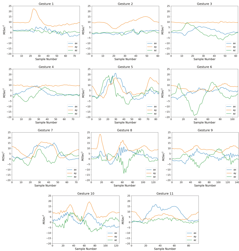
Figure 14. Samples of waveforms produced by accelerometers in three axes (gx, gy, and gz) for each gesture.
