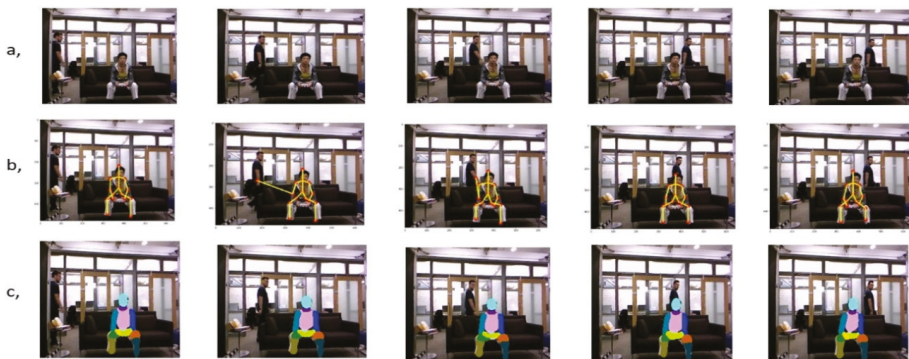
Figure 1. Illustration of the case in which many actors are present in the scene. The first row (a) RGB input images, the second row (b) extracted skeleton joints images, and the last row (c) color-encoded body part segmentation images. In this case, the skeleton joints extraction can be distracted by other objects in the background, but the color-encoded body part segmentation can help avoiding such a case.
