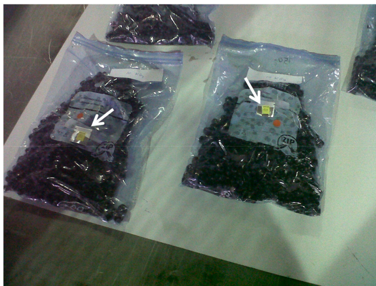
Figure 11. Red grapes in plastic bags after e-beam irradiation. The white arrows indicate the location of radiochromic dosimeters.
