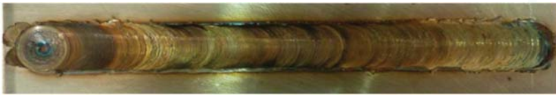
Figure 2. Surface morphology of friction stir welding (FSW) butt joint.
