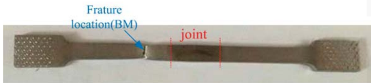
Figure 11. The macro pictures of the failure in the BM.
