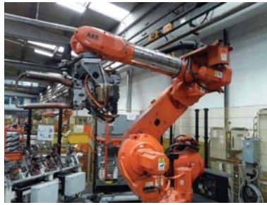
Figure 4. The medium-frequency direct current (MFDC) resistance spot-welding (RSW) machine connected to the ABB robot arm used in this investigation.
