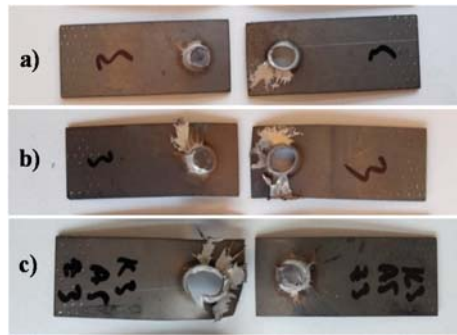
Figure 20. The fracture modes of the tensile shear test samples: (a) 9 kA; (b) 11 kA; (c) 12 kA.
