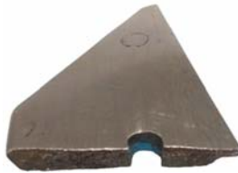
Figure 4. Broken share-point part made of pearlitic steel.
