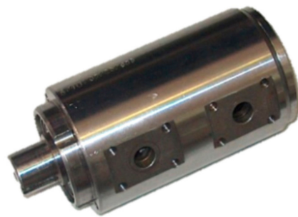
Figure 8. General view of hydraulic satellite motor (SM type) [30].
