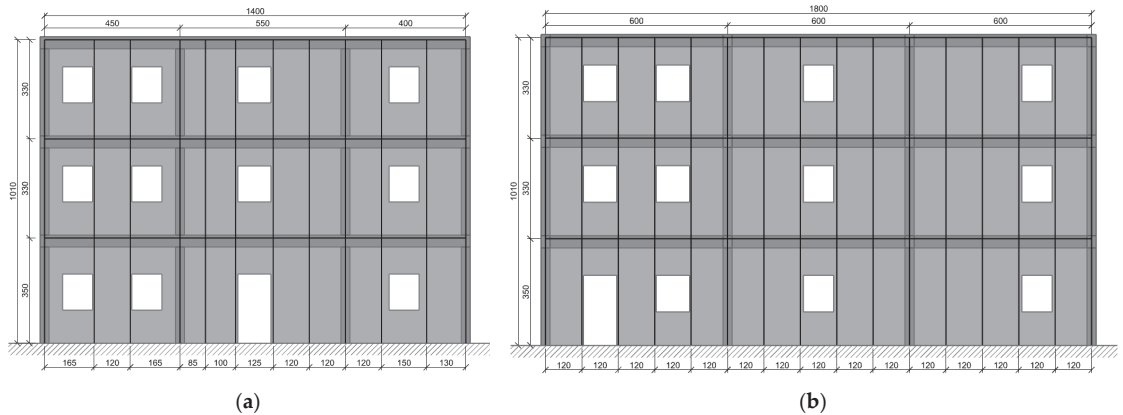
Figure 9. RC-framed skin applied to the existing RC building with evidenced the opening lay-out: (a) transversal view; (b) longitudinal view.
