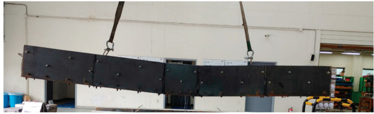
Figure 11. The shape of the test specimen after a flexural test.
