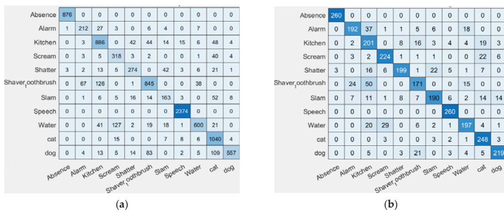
Figure 5. Confusion matrices for the top performing algorithm—CWTFT scalograms for: (a) Imbalanced dataset using the full synthetic database; (b) balanced dataset with 1565 files for training, and 260 files for testing.
