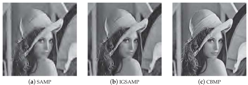
Figure 6. Reconstructed results of the Lena image by SAMP, IGSAMP, and CBMP with the initial step size of 64.
