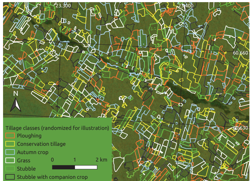
Figure 1. Foreground polygons: Autumn tillage operations annotated to six classes (colors). Background raster: Red-green rendering of a VH+VV dual polarization Sentinel-1 SAR image. Note: Due to data protection regulations, the polygons are from publicly open similar data from 2016 instead of our actual data, and the classes are randomized.
