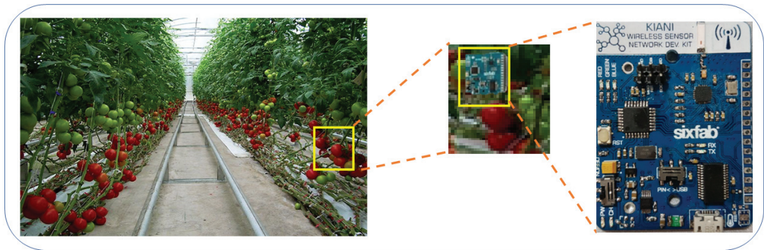
Figure 2. The device used as an IoT node in the field [5,55].
