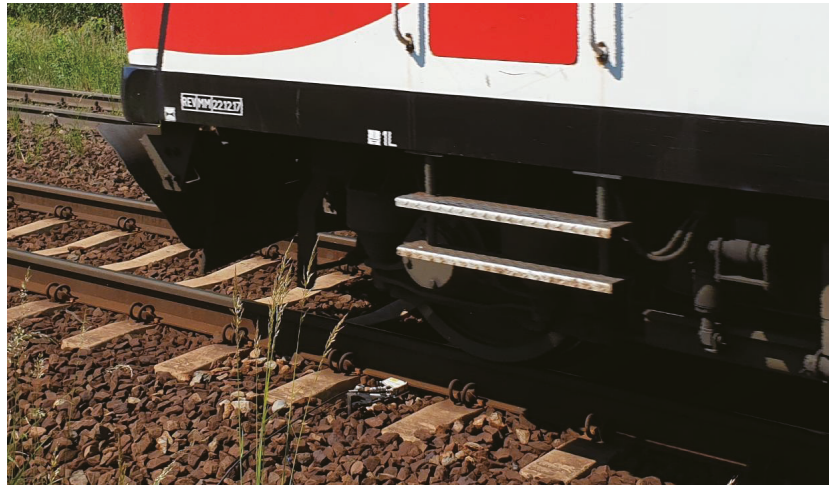
Figure 8. Railway viaduct at km 83,808 LK No. 272—measurement of the vertical displacement of a rail dynamically loaded with a train of Koleje Wielkopolskie.
