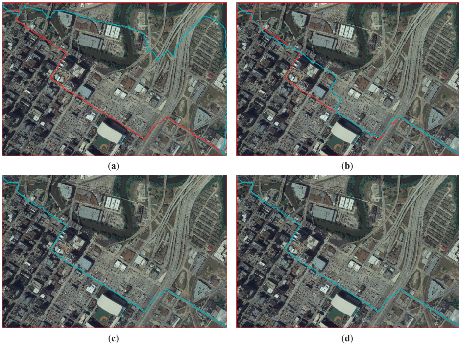
Figure 11. Experiments of seamline determination for Dataset A with different values of w : (a) w is 0.001 (red line) and w is 0.1 (cyan line), (b) w is 0.001 (red line) and w is 0.01 (cyan line), (c) w is 0.001 (red line) and w is 0.0001 (cyan line), and (d) w is 0.001 (red line) and w is 0.00001 (cyan line).
