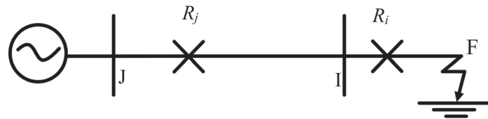
Figure 1. A single-end radial distribution system.
