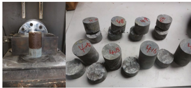
Figure 11. Equipment and failure modes of direct shear test.
