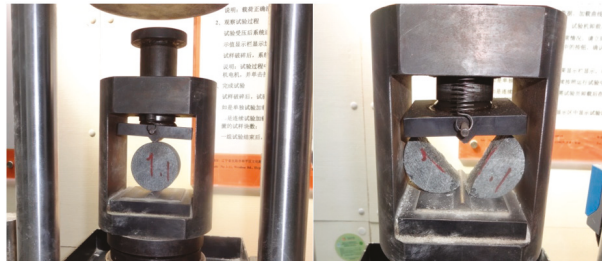
Figure 10. Equipment and failure modes of Brazilian splitting test.
