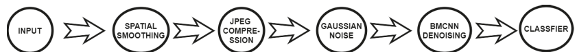
Figure 7. A defensive pipeline which utilises all the researched defences, except total variance minimisation.
