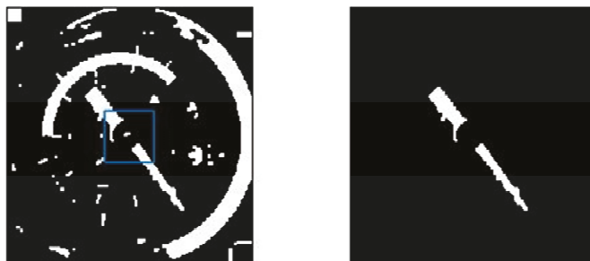
Figure 12. The situation of the broken pointer.
