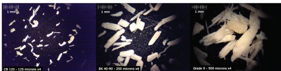
**Figure 1.** From left to right, micrographs of CB 120 retained on the sieve of 125 microns, BK 40-90 retained on the sieve of 250 microns and Grade 9 retained on the sieve of 500 microns.
