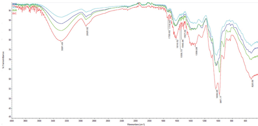
Figure 3. Fourier-transform infrared spectroscopy spectra of red beetroot dried samples: BV C , BC C —red beet purée dried by convection method; BV IR , BC IR —red beet purée dried by infra-red (IR) method.
