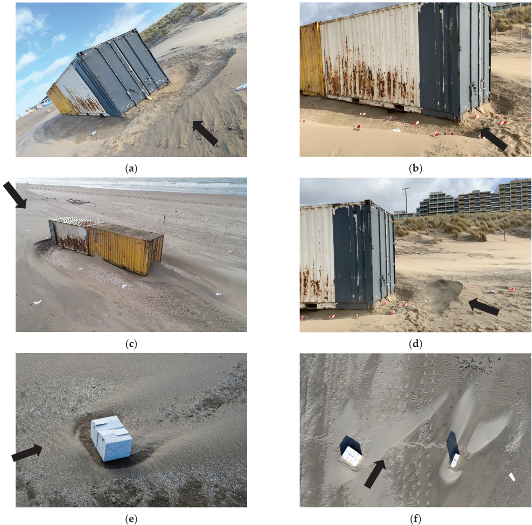
Figure 9. Field observations of erosion and deposition patterns around a (a–d) full-scale model at Noordwijk beach, and (e,f) small-scale models at De Zandmotor beach, the Netherlands. The arrows show the wind directions. (c,e,f were obtained from Poppema et al. [18]).
