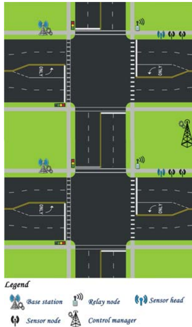
Figure 5. Major components of the proposed architecture.
