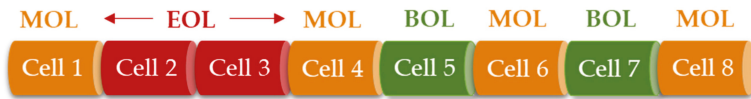
Figure 11. Mixed aging scenario for cell-to-cell variations considered for the 8S module in this study [14].
