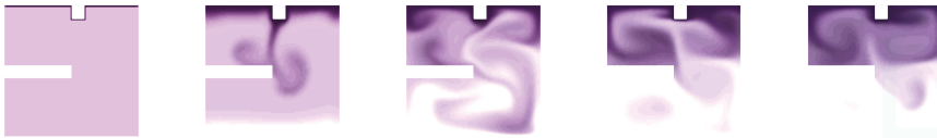
(c) Hot Room (resolution 101 \times 101 , 265 time steps): air flow within a closed container, driven by buoyant forces imposed by a heated bottom plate and a cooled top plate. To provoke transient aperiodic flow, the container exhibits two barriers (one on the top, one on the bottom).
