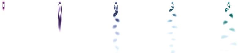
(b) von Kármán (resolution 301 \times 101 , 418 time steps): 2D time-dependent CFD simulation of a von Kármán vortex street.
