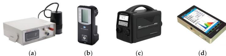
**Figure 4.** Testing devices for lighting environment parameters in tunnel. (a) Reflectance tester, (b) illuminance meter, (c) luminance meter, (d) multifunctional spectrometer.
