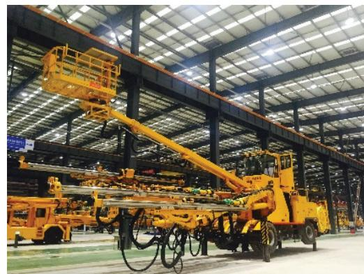
**Figure 3.** Intelligent drill jumbo (made by China Railway Construction Heavy Industry Corporation Limited).
