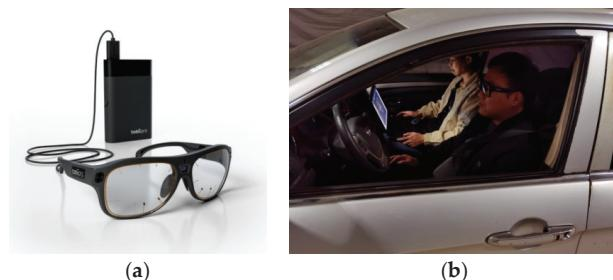
**Figure 6.** Acquisition of a driver's pupil diameter data. (a) Eye tracker, (b) the driver wearing eye tracker.
