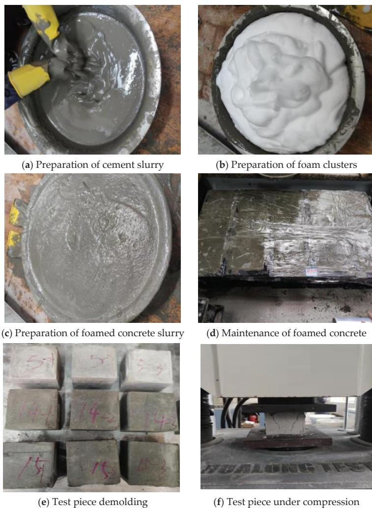
Figure 8. Schematic of test.
