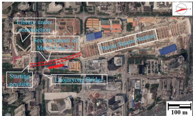
Figure 23. Surrounding environment of section tunnel project.
