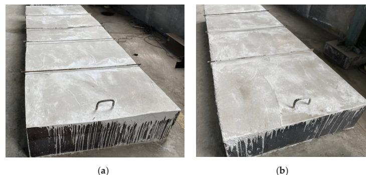
**Figure 4.** After pouring of the spatial reticulated grid components. (a) The BEJC50 × 6 component and (b) the JSC50 × 6 component.
