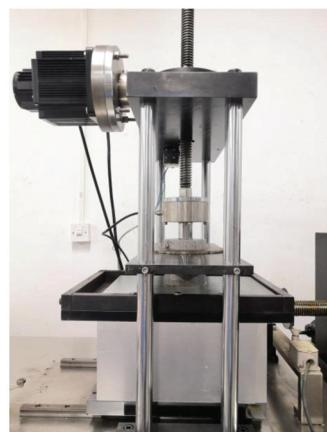
**Figure 3.** Physical drawing of the direct shear test.
