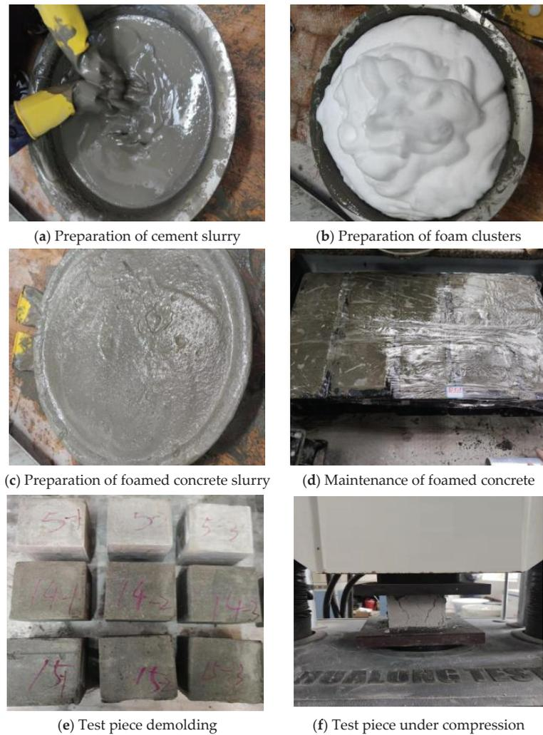
Figure 8. Schematic of test.
