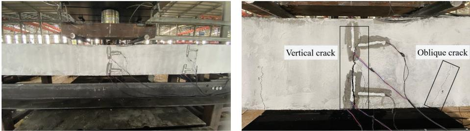
Figure 7. Failure characteristics of the BEJC50 × 6 component.
