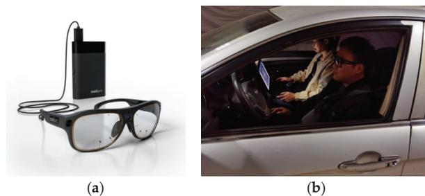
Figure 6. Acquisition of a driver’s pupil diameter data. (a) Eye tracker, (b) the driver wearing eye tracker.
