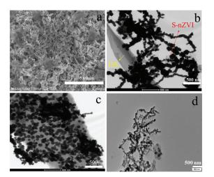
Figure 2. (a) SEM image of S-nZVI@OS; (b,c) TEM images of S-nZVI@OS; (d) TEM image of S-nZVI@OS after reaction.
