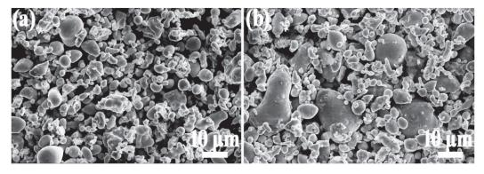
Figure 4. Comparison of Fe-Si-Cr powders: (a) Fe-Si-Cr raw powder, (b) Fe-Si-Cr phosphated powder.
