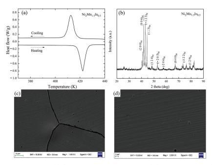
**Figure 3.** (a) DSC curve [30], (b) XRD pattern at room temperature [30], (c,d) microstructures of Ni<sub>2</sub>Mn<sub>1.5</sub>In<sub>0.5</sub> alloy.
