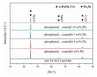
Figure 8. XRD patterns of Fe-Si-Cr powders with different PI coating contents.
