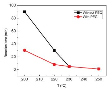
**Figure 2.** Reaction time dependence on the temperature maintained by the microwave reactor. A difference is noticed in the reaction times at low temperatures when PEG is added to the initial reaction mixture.
