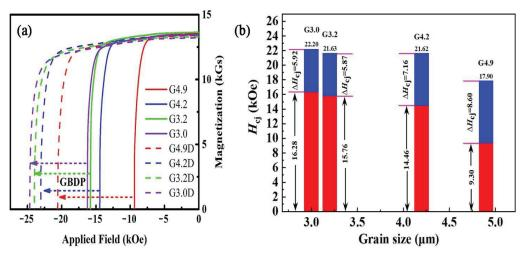
**Figure 2.** (a) The demagnetization curves of the original magnets (G4.9, G4.2, G3.2, and G3.0) and the diffused magnets (G4.9D, G4.2D, G3.2D, and G3.0D) with different grain sizes; (b) the coercivity of magnets with different grain sizes before and after the diffusion process (the red bars represent  $H_{cj}$  for the original magnets, and the blue bars represent the increments of  $H_{cj}$  after the diffusion process).
