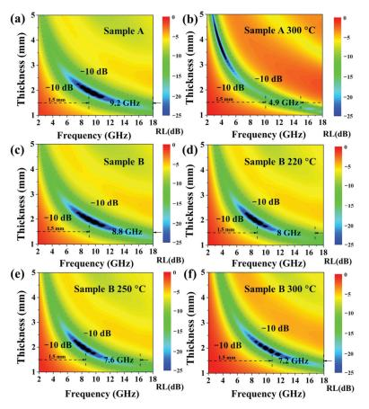
**Figure 5.** Reflection loss (RL) maps of sample A (a), sample A annealing at 300 °C (b), sample B (c), sample B annealing at 220 °C (d), sample B annealing at 250 °C (e), and sample B annealing at 300 °C (f).
