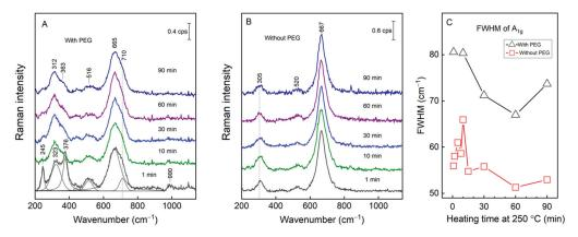
**Figure 4.** Raman spectra of the samples prepared with (**A**) and without (**B**) PEG heated from 90 to 1 min. The dependence of the full width at half maximum (FWHM) of the  $A_{1g}$  mode on the MPs preparation time at 250 °C with (black triangles) and without (red squares) PEG (**C**). The excitation wavelength was 830 nm; the laser power was set to 0.8 mW; the acquisition time was 60–120 min.
