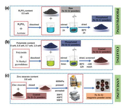
**Figure 1.** The preparation process of Fe-Si-Cr@PI core–shell structure coating and magnetic powder cores: (**a**) phosphating, (**b**) coating, and (**c**) annealing.
