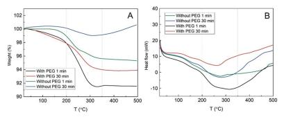
**Figure 7.** TGA data of samples synthesized with PEG and without PEG; synthesis time—1 or 30 min at 250 °C. Changes in sample weight (**A**) and heat flow (**B**) are registered from room temperature to 500 °C.
