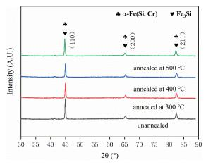
Figure 11. XRD patterns of Fe-Si-Cr SMCs at different annealing temperatures.
