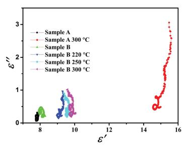
**Figure 7.** Typical Cole–Cole semicircles of  $\varepsilon'$  vs.  $\varepsilon''$  for sample A and B before and after annealing.
