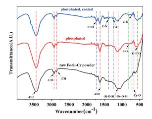
Figure 7. FTIR spectrum of uncoated and coated Fe-Si-Cr powder (from bottom to top is the raw powder, phosphated powder, and phosphate-coated powder.
