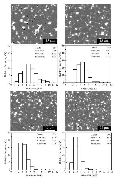
Figure 1. BSE SEM images and corresponding grain size distributions after sintering of magnetic powders with different particle sizes, (a) G4.9, (b) G4.2, (c) G3.2, (d) G3.0.
