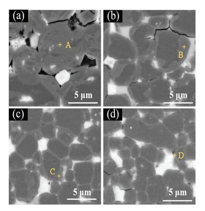
Figure 5. The BSE-SEM images at 15  $\mu$ m from the surface of (a) G4.9D, (b) G4.2D, (c) G3.2D, and (d) G3.0D diffused magnets.
