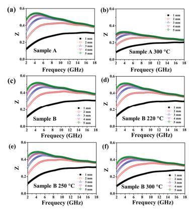
**Figure 6.** The impedance matching value Z of sample A (a), sample A annealing at 300 °C (b), sample B (c), sample B annealing at 220 °C (d), sample B annealing at 250 °C (e), and sample B annealing at 300 °C (f).
