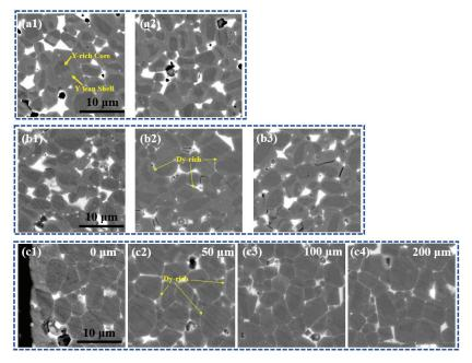
**Figure 3.** The microstructures of the original magnet,  $DyH_x$  addition magnet, and the  $DyH_x$  diffusion magnet. (**a1,a2**) are two different positions of the original magnet, (**b1–b3**) are three random positions in the  $DyH_x$  addition magnet, and (**c1–c4**) are the microstructures at the depths of 0  $\mu$ m, 50  $\mu$ m, 100  $\mu$ m, and 200  $\mu$ m from the surface of the  $DyH_x$  diffusion magnet, respectively.
