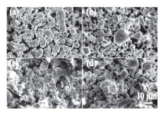
Figure 6. Fe-Si-Cr powders coated with PI: (a) 0 wt% PI, (b) 0.4 wt% PI, (c) 0.7 wt% PI, (d) 1.0 wt% PI.
