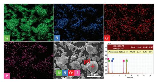
Figure 5. The EDS of Fe-Si-Cr phosphated powder.
