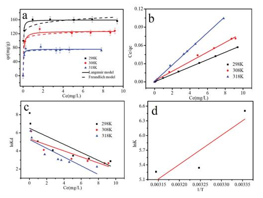
**Figure 7.** (a) Adsorption isotherms for Cr (VI) on S-nZVI@OS at 298, 308 and 318 K; (b) Langmuir plot; (c) linear plots of  $\ln K_d$  versus  $C_e$ ; (d) linearized Arrhenius plot of  $\ln K$  as a function of 1/T.
