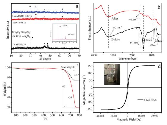
**Figure 4.** (a) XRD patterns of different composite before and after removal Cr (VI) (inset figure is the XRD pattern of OS after reaction with Cr (VI)); (b) FTIR spectra of S-nZVI@OS before and after reaction; (c) TG thermogram of OS and S-nZVI@OS; (d) magnetization curve of S-nZVI@OS.
