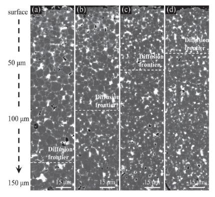
**Figure 3.** The longitudinal cross-sectional BSE-SEM images of (**a**) G4.9D, (**b**) G4.2D, (**c**) G3.2D, and (**d**) G3.0D diffused magnets.
