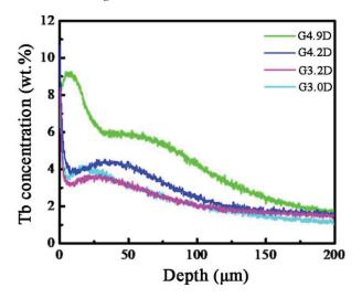
Figure 4. Tb contents as a function of depth from the surface of G4.9D, G4.2D, G3.2D, and G3.0D diffused magnets.
