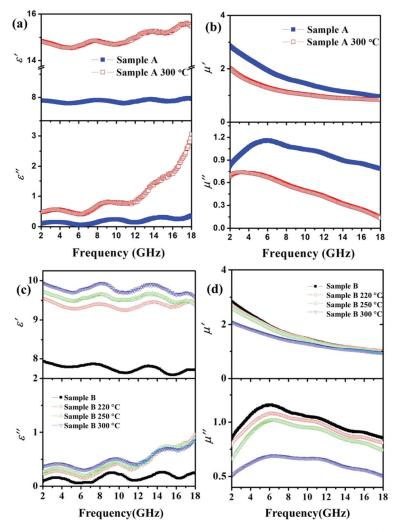
**Figure 4.** The permittivity spectra (**a**) and permeability spectra (**b**) of sample A before and after annealing at 300 °C; the permittivity spectra (**c**) and permeability spectra (**d**) of sample B before and after annealing at 220 °C, 250 °C, and 300 °C.
