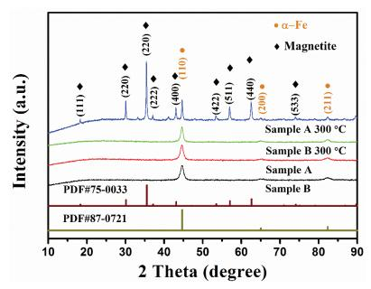
Figure 2. The XRD patterns of samples A and B before and after annealing at 300 °C.
