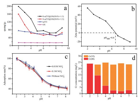
**Figure 6.** (a) The adsorption capacity of OS, nZVI and S-nZVI@OS for Cr (VI) under different initial pH; (b) Zeta potential of S-nZVI@OS; (c) Effect of ionic strength at different initial pH on Cr (VI) removal; (d) residual concentration of total Cr, Cr (VI) and Cr (III) after reaction in solution.
