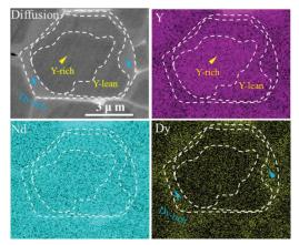
Figure 5. Back-scattered SEM image mappings for the  $DyH_x$  diffusion magnet at the depth of 50  $\mu$ m.
