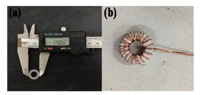
Figure 2. The SMCs sample to be tested: (a) magnetic powder core size and (b) coil winding before magnetic performance test.
