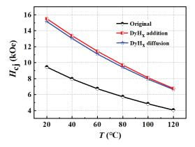
Figure 6. The coercivity versus temperature of the original magnet, the  $DyH_x$  addition magnet, and the  $DyH_x$  diffusion magnet.
