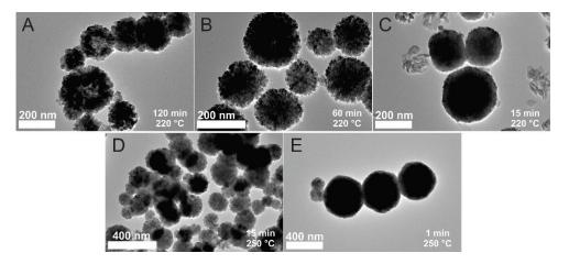
**Figure 5.** TEM images of the synthesized samples without PEG: 220 °C, 120 min (**A**); 220 °C, 60 min (**B**); 220 °C, 15 min (**C**); 250 °C, 15 min (**D**); 250 °C, 1 min (**E**). The scale bar for (**A**–**C**) is 100 nm, and the scale bar for (**D**) and (**E**) is 200 nm.
