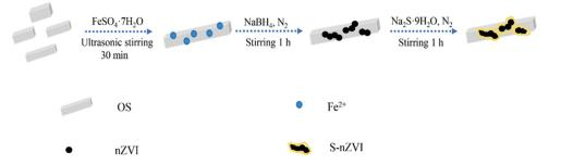
Figure 1. Schematic diagram of S-nZVI@OS synthesis.
