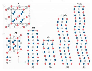
Figure 1. Crystal structures of (a) cubic austenite, (b) NM martensite, (c) 5M martensite, (d) 6M martensite, (e)  $7M - (5\overline{2})_2$  martensite, and (f) 7M–IC martensite for Ni<sub>2</sub>MnIn alloy.
