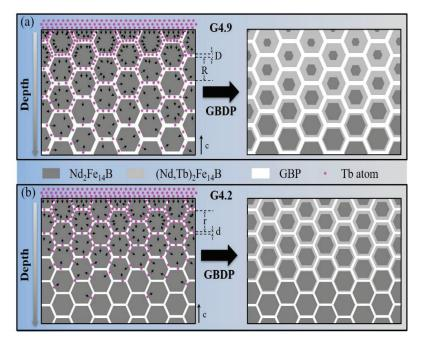
Figure 6. The schematic illustration of the diffusion process of the (a) G4.9 and (b) G4.2 magnets.
