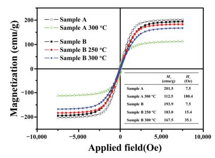
Figure 3. The hysteresis loops of samples A and B before and after annealing at 250 °C and 300 °C.
