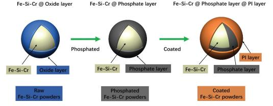
Figure 3. The effect of phosphating and coating process on the surface of Fe-Si-Cr powder particles.
