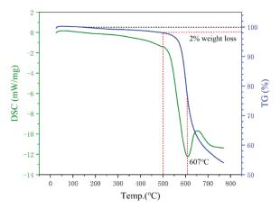
Figure 10. Kinetic curves of thermal decomposition of PI in argon.
