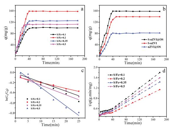
**Figure 5.** (a) The adsorption kinetics of Cr (VI) with different S/Fe ratios; (b) the adsorption kinetics of S-nZVI, nZVI@OS and S-nZVI@OS; (c) Liner polts of  $\ln C_t/C_0$  versus T; (d) pseudo-second-order dynamics diagram.
