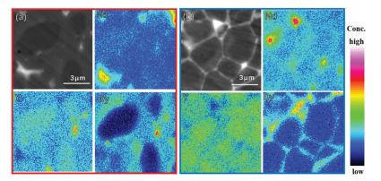
Figure 4. EPMA elemental mappings of the  $DyH_x$  addition magnet (a) and the  $DyH_x$  diffusion magnet (b).
