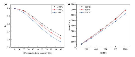
**Figure 12.** The trend of magnetic properties with annealing temperature (the powder was phosphated and coated with 0.4 wt% PI): (**a**) relative permeability; (**b**) core loss.
