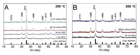
**Figure 3.** XRD diffractograms of Fe<sub>3</sub>O<sub>4</sub> particles at synthesis temperatures of 250 °C (**A**) and 200 °C (**B**). The diffractograms of different synthesis times are presented, as well as a presence of PEG in the reaction mixture.
