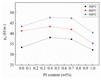
Figure 13. Trend of PI content and annealing temperature on effective permeability of Fe-Si-Cr SMCs.
