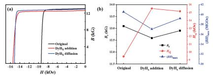
**Figure 1.** (a) The demagnetization curves of the original magnet, the  $DyH_x$  addition magnet, and the  $DyH_x$  diffusion magnet; (b) the variation curves of the corresponding  $B_r$ ,  $H_{cj}$ , and  $(BH)_{max}$  of the three types of magnets derived from (a).
