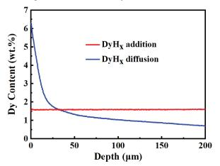
Figure 2. The Dy concentration distributions of the  $DyH_x$  addition and diffusion magnets in the depth range of 0–200  $\mu$ m.
