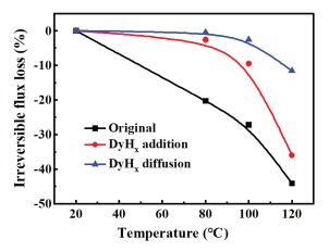
Figure 7. Irreversible loss of flux versus temperature of the original magnet, the  $DyH_x$  addition magnet, and the  $DyH_x$  diffusion magnet.
