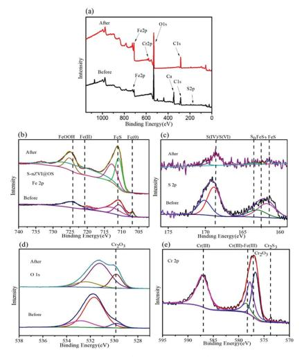
**Figure 9.** (a) XPS survey of S-nZVI@OS before and after reaction with Cr (VI); (b) Fe2p spectra before and after reaction; (c) S2p spectra before and after reaction; (d) O1s spectra before and after reaction; (e) Cr2p spectrum.
