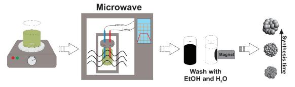
Figure 1. Synthesis scheme of Fe<sub>3</sub>O<sub>4</sub> submicron spheres.
