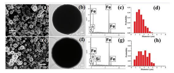
**Figure 1.** Scanning Electron Microscope (SEM) (**a**) and Transmission Electron Microscope (TEM) (**b**) images of sample A, EDS spectrum of sample A for the selected area (**c**), and particle size distribution of sample A (**d**); SEM (**e**) and TEM (**f**) images of sample B, EDS spectrum of sample B for the selected area (**g**), and particle size distribution of sample B (**h**).
