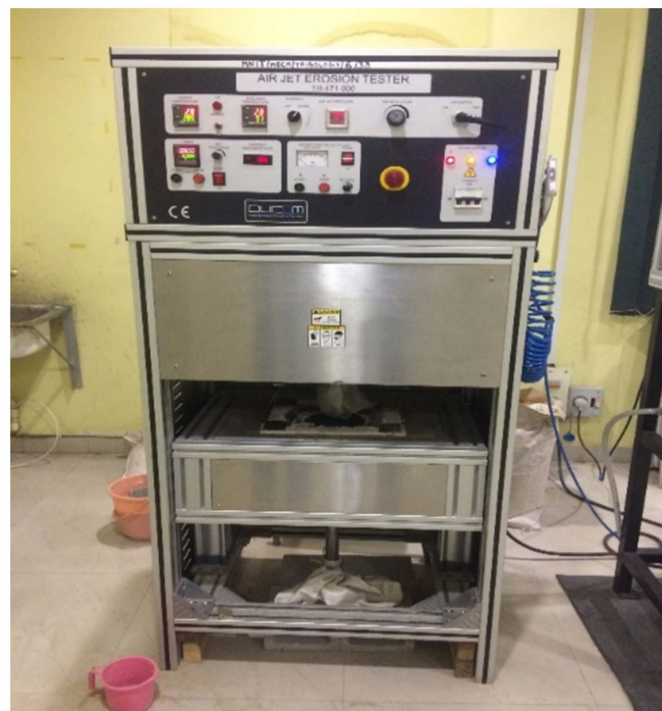
Figure 5. Air jet erosion test machine set up.
