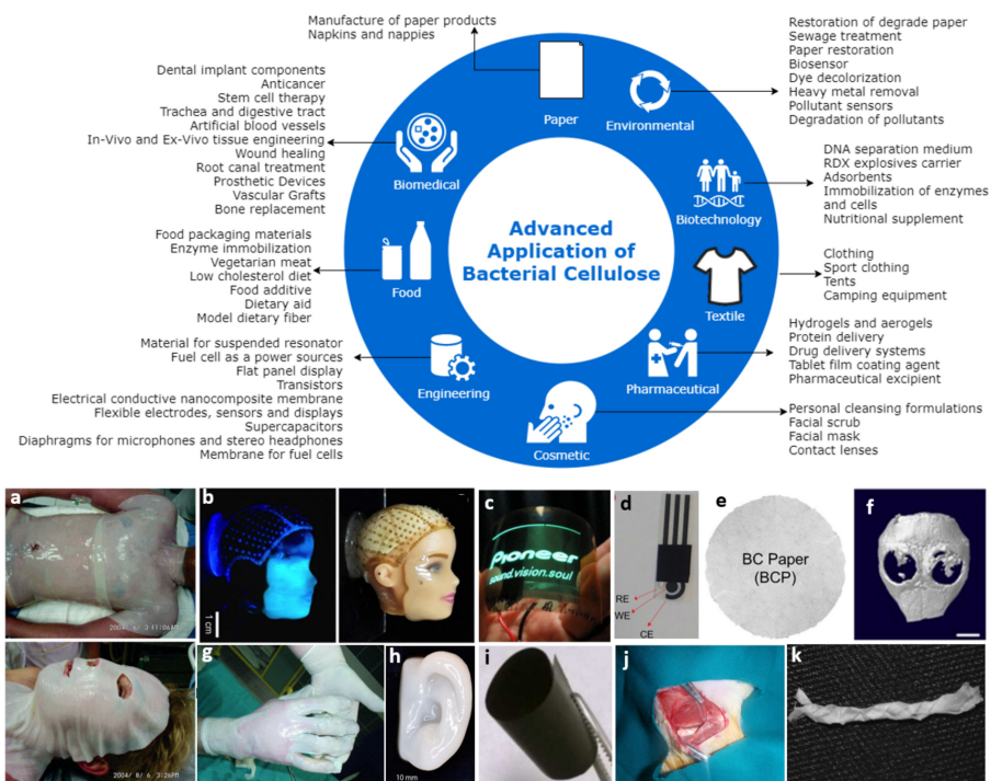
Figure 4. Advanced application of bacterial cellulose (BC). (a) A never-dried microbial cellulose membrane shows remarkable conformability to the various body contours, maintains a moist environment, and significantly reduces pain [74]. (b) A doll face was scanned, and a 4.5 wt % Flink containing A. xylinum was deposited onto the face using a custom-built 3D printer. In situ cellulose growth leads to the formation of a cellulose-reinforced hydrogel that, after removal of all biological residues, can serve as a skin transplant [75]. (c) Luminescence of an organic light-emitting diode deposited onto a flexible, low-CTE, and optically transparent cellulose nanocomposite [76]. (d) Screen-printed electrodes made on BC substrate [77]. (e) BC paper [78]. (f) Bone regeneration efficacy of the scaffolds [79]. (g) Microbial cellulose dressing applied on a wounded hand [80]. (h) 3D Bioprinting Human Chondrocytes with nanocellulose–alginate bioink [81]. (i) Flexible freestanding nanocellulose paper-based Si Anodes for Lithium-ion batteries [82]. (j) Cellulose acetate/poly lactic acid coaxial wet-electrospun scaffold containing citalopram-loaded gelatin nanocarriers for neural tissue [83]. (k) Artificial Bacterial cellulose ligament or tendons [84].
