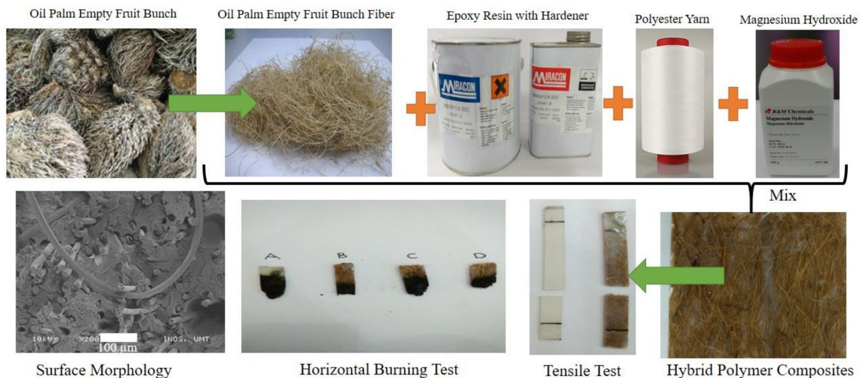
Figure 5. Extraction of OPEBF, and fabrication of OPEBF/polyester yarn, magnesium hydroxide reinforced epoxy resin hybrid composite. Extracted from [69] with permission.
