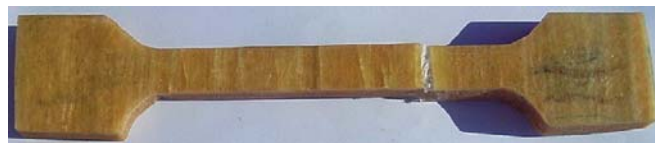
Figure 9. Tensile specimen fracture mode.
