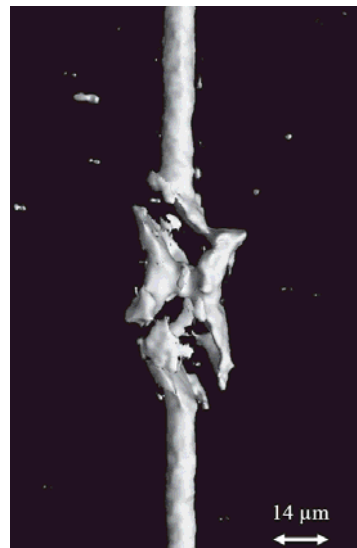
Figure 5. Example of one 3D location of fiber fracture image in high-resolution, taken by XRM, allowing the measurement of the inclination angle of the fracture planes and the size of the small fracture pieces between single fragments.
