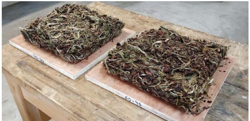
Figure 4. Particleboards made from varying mixtures of tree bark and hemp fibers (70:30 left and 60:40 right).
