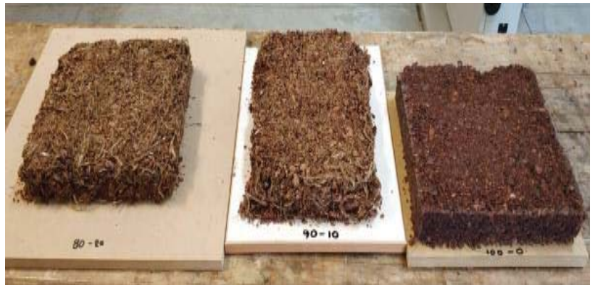
Figure 5. Particleboards made from varying mixtures of tree bark and hemp fibers (80:20 left and 90:10 center) and panels consisting only of bark (right).
