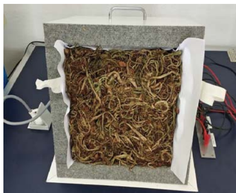
Figure 6. The EI-700 unit “box method” for the thermal conductivity measurements.
