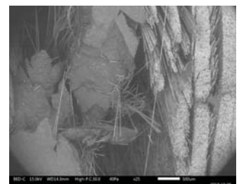
Damaged sample at 4 bar
