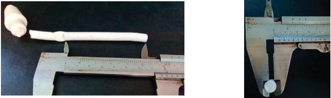
Figure 4. Cracked specimen for fretting ring distance above 70 mm (left), and deformed diameter (right).
