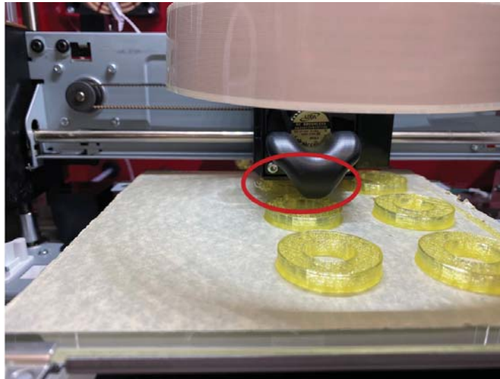
Figure 6. Nozzle blockage fault in a 3D printing machine.
